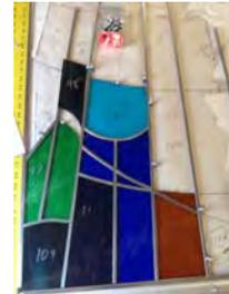
The next step will be to solder the came and then clean the solder flux off the glass.
